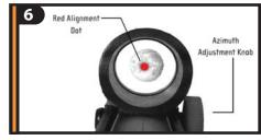
With the object centered in the eyepiece, use the azimuth (right/left) and altitude (up/down) adjustment knobs on the finderscope to place the red alignment dot directly over the centered object.
